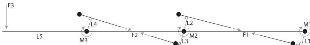
Figure 13, M_1 , M_2 and M_3 are the torque of the joints. F_1 and F_2 are the forces in the bending linkages (red linkages in figure 12). F_3 is an external force at the tip of the finger. L_1 , L_2 , L_3 , L_4 and L_5 are the lever arms to the joints.
