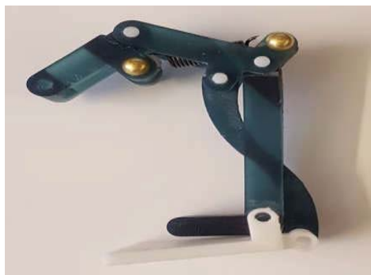
Figure 16, Second prototype. Side view, flexed finger
