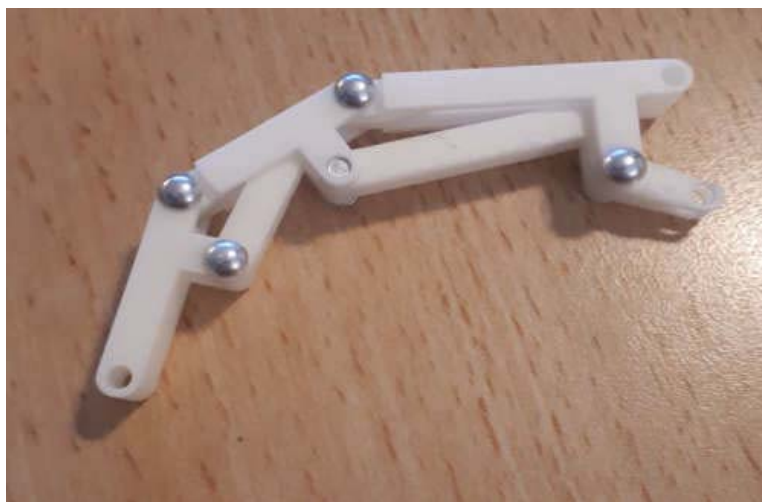
Figure 11, The second finger design as it was derived, here 3D printed and assembled.
